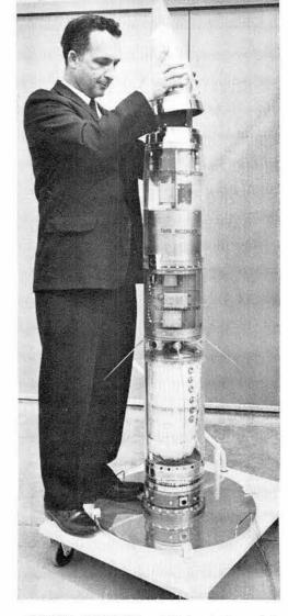
TYPICAL PAYLOAD — Nitehawk 9 model payload section is examined by W. C. Womack, project engineer for the sounding rocket system. Instead of the conventional metal casing, this demonstration section is covered with plastic to show the location of typical payload components which are labeled for briefing purposes.
